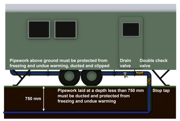
Installation or alteration of any pipework laid at less than 750 mm or above ground, even when the work is undertaken by an approved contractor is always notifiable. For further information speak to the local water undertaker.
