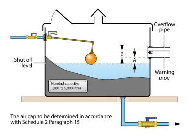
'A' is 25 mm and is the level at which audible or visible alarm is activated 'B' is not less than 50 mm between invert of overflow pipe and shut off level
