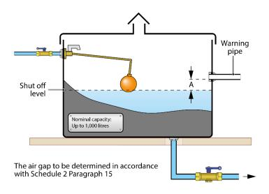
'A' and 'B' are not less than 25 mm
