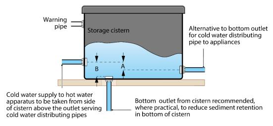
'A' or 'B' to be not less than internal diameter of outlet of cold water distributing pipe
