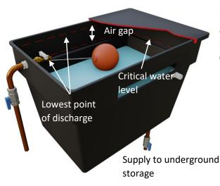
In the case of wholesome water applications, the overflow should be fitted with a screen and light cowl
