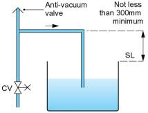
'Type DA – Anti-vacuum valve (or vacuum breaker)' means a mechanical backflow prevention device with an air inlet which is closed when water within the device is at or above atmospheric pressure but which opens to admit air if a vacuum occurs at the inlet to the device.
