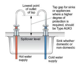
Type AUK3 – Higher risk tap gap' means the height of an air gap between the lowest part of the outlet of a tap, combination fitting, shower head or other fitting discharging over any appliance or other receptacle, and the spillover level of that appliance, where a fluid category 4 or 5 risk is present downstream.
