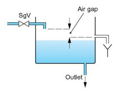
'Type AF – Air gap with circular overflow' means a non-mechanical backflow prevention arrangement of water fittings with an air gap measured downwards from the lowest point of the discharge orifice, which discharges into the receptacle, to the critical level.
