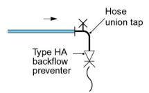
'Type HA – Hose union backflow preventer' means a mechanical backflow prevention device for fitting to the outlet of a hose union tap and consisting of a single check valve with air inlets that open if the flow of water ceases.
