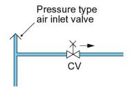
'Type LA – Pressurised air inlet valve' means an anti-vacuum valve or vacuum breaker, similar to Type DA but suitable for conditions where the water pressure at the outlet of the device under normal conditions of use is greater than atmospheric.
