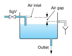
'Type AC – Air gap with vented submerged inlet and circular overflow' means a non-mechanical backflow prevention arrangement of water fittings with a vented, but submerged, inlet; the air gap being measured vertically downwards from the lowest point of the air inlet to the critical level.
