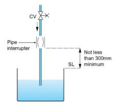
'Type DB – Pipe interrupter with atmospheric vent and moving element' means a mechanical backflow prevention device with an air inlet closed by a moving element when the device is in normal use but which opens and admits air if the water pressure upstream of the device falls to atmospheric pressure, the device being installed so that the flow of water is in a vertical, downward direction.
