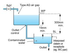
'Type AUK1 – Air gap with interposed cistern' means a non-mechanical backflow prevention arrangement consisting of a cistern with a Type AG overflow and an air gap; the spill-over level of the receiving vessel (WC pan or other receptacle) being located not less than 300 millimetres below the overflow pipe and not less than 15 millimetres below the lowest level of the interposed cistern.
