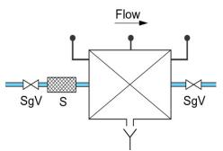
'Type BA – Verifiable backflow preventer with reduced pressure zone' means a verifiable mechanical backflow prevention device consisting of an arrangement of water fittings with three pressure zones with differential obturators and that will operate when potential backflow conditions obtain or there is a malfunction of the valve.
