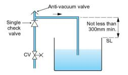
'Type DUK1 – Anti-vacuum valve combined with a single check valve' means a mechanical backflow prevention device comprising an anti-vacuum valve with a single check valve located upstream.
