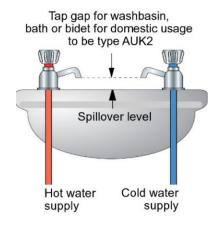
'Type AUK2 – Domestic tap gap' means the height of air gap between the lowest part of the outlet of a tap, combination fitting, shower head or other fitting discharging over a domestic sanitary appliance or other receptacle, and the spillover level of that appliance, where a fluid category 2 or 3 risk is present downstream.
