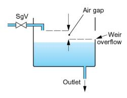
'Type AB – Air gap with weir overflow' means a non-mechanical backflow prevention arrangement of water fittings complying with Type AA, except that the air gap is the vertical distance from the lowest point of the discharge orifice which discharges into the receptacle, to the critical water level of the rectangular weir overflow.
