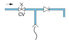
'Type HC – Diverter with automatic return' means a mechanical backflow prevention device used in bath/shower combination tap assemblies which automatically returns the bath outlet open to atmosphere if a vacuum occurs at the inlet to the device.
