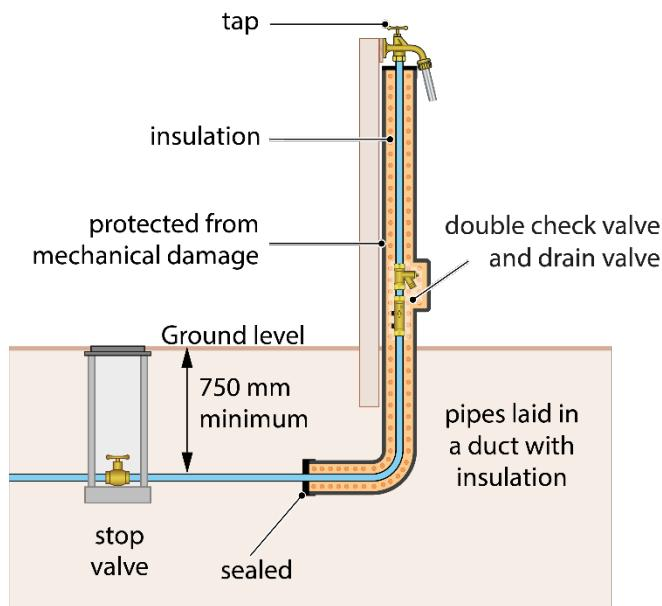
The image opposite is an example of what might be an acceptable building standpipe arrangement. Please note the double check valve is providing wholesite rather than point of use backflow protection.
